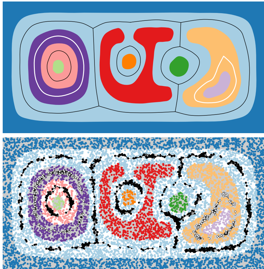
Figure 33: Expected and observed regions as well as Voronoi boundaries for the complex areal object originally displayed in Figure 25. Black and white lines represent the Voronoi boundaries induced by positive and negative region components respectively. Displays an example implementation of modules 1 and 2 on a network with 10,000 nodes.
